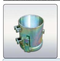
Used to determine the degree of compaction of asphalt for road pavement quality control testing. The unit consists of a mould split vertically on one side together with a clamp-attached baseplate. Plated for protection against corrosion.
