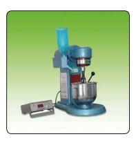
■ Laboratory mixer 5 litres capacity complete with whisk.
